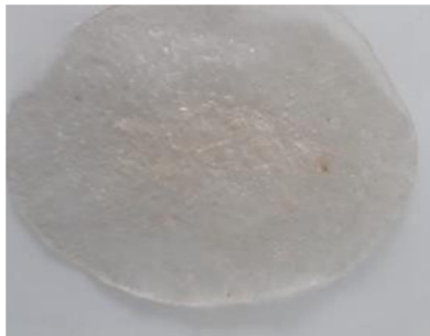
Gambar 2. Edible film glukomanan umbi porang
